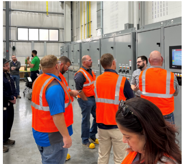
In the photo above, a long section of paralleling switchgear is tested at the Kohler factory with generators in the next room.
